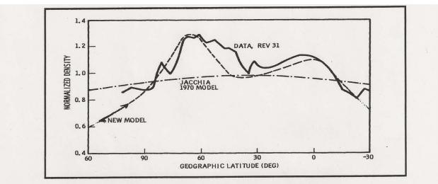
Densities measured by the accelerometer on LOGACS near 180 km and the Jacchia 1970 model versus geographic latitude. This shows that models based on orbital decay measurements average out the atmospheric variability when the orbital eccentricity is moderate (which is the typical case).
